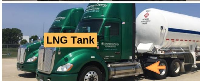
An LNG fuel system enables an 800+ mile range for a day-cab. This range is ideal for hub-and-spoke transportation networks, where trucks are domiciled and return to their hub after one to two days.
